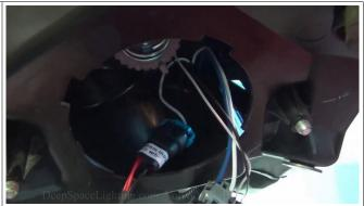
14. Connect single-pin wires from ballast to bulb adapter leads, and connect adapter harness *Ballast* connector to ballast input.
