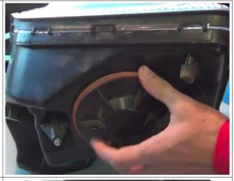
4. Loosen the E6 (external Torx) aim adjusting screw several turns and lubricate if there are any signs of corrosion on it to make adjustment easier.
