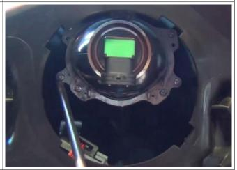
7. Remove projector through bulb access hole.
