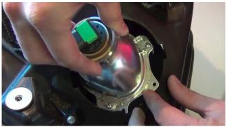
8. Remove bulb retaining nut and spring from bixenon projector. Remove xenon bulb from Do not touch the glass surface. If you do, or There is a locating tab on both the bulb to orient the bulb properly. Re-install spring and should be cleaned with an alcohol wipe. bulb retaining nut.
