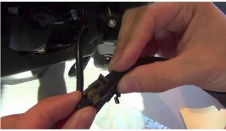
15. Connect bulb adapter to xenon bulb by aligning tabs on bulb, and twisting clockwise until locked. Do not use excessive force.
