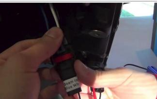
12. Connect adapter harness *High Beam Solenoid* connector to the connector attached to the bixenon projector (small red and black wires). Make sure connectors are inserted straight to avoid bending pins.
