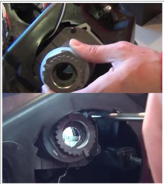
11. Connect Low Beam Input connector on adapter harness to connector removed from low beam bulb in step 9. Verify that plug is oriented correctly.
