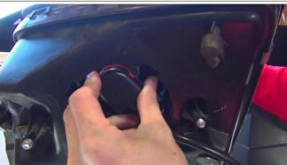
16. Secure ballast inside headlamp housing and reinstall headlamp housing onto hood. Reconnect headlamp harness to vehicle harness, and confirm headlamp operation with engine running.
