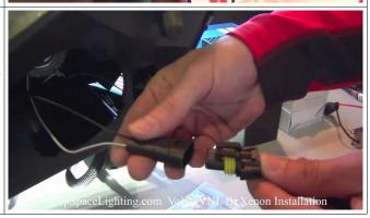
13. Unplug headlamp harness from high beam (lower) bulb, and connect the plug removed from the high beam bulb to the High Beam Input connector on the adapter harness.
