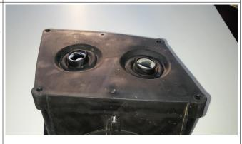
5. Lift around the edges of the rubber cover to remove.
