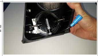
8. Lay the rubber housing back in place, and pull fog light wires through lower opening. Slide grommet over wires and insert into the hole for the fog light bulb to seal the opening.
