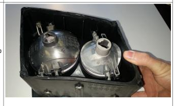
6. Carefully remove the fog light reflector by lifting up on the pin furthest from the adjuster first. Be careful not to apply sideways pressure on the housing's clips—they can be broken easily.
