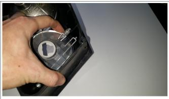
7. Insert aiming tab into the fog light adjuster, and snap both mounting bolts into the housing's clips.
