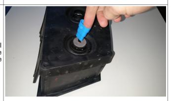
9. Connect fog light plug to the original fog light plug (yellow and black wires on OE harness).
