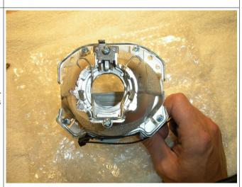
13. Set new projector in frame, and mount in place using screws removed in step 10.
