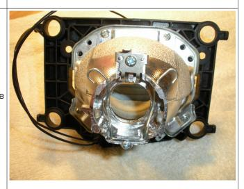
14. Enlarge low beam wiring access hole to 1-1/2" diameter. Test fit grommet on ignitor wiring. Clean any loose material from housing before proceeding.
