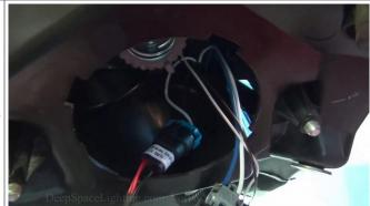
24.Connect bulb to ballast connector to ballast and bulb, and connect adapter harness *Ballast* connector to ballast input.
