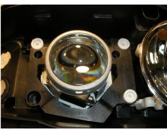
16. Install projector shroud by pushing it onto projector. Reinstall large shroud with 4 screws removed in step 7.
