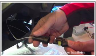
23. Unplug headlamp harness from high beam bulb, and connect the plug removed from the high beam bulb to the *High Beam Input* connector on the adapter harness. Optionally, reconnect high beam bulb using connector labeled *High Beam*.
