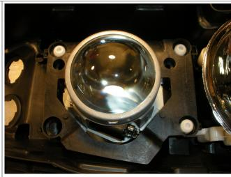
15. Set frame back in housing, and reinstall retaining rings.
