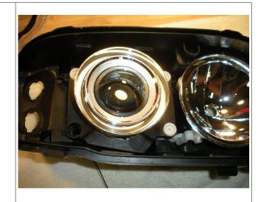
9. Remove 3 adjuster retaining rings by prying up with a small flathead screwdriver.
